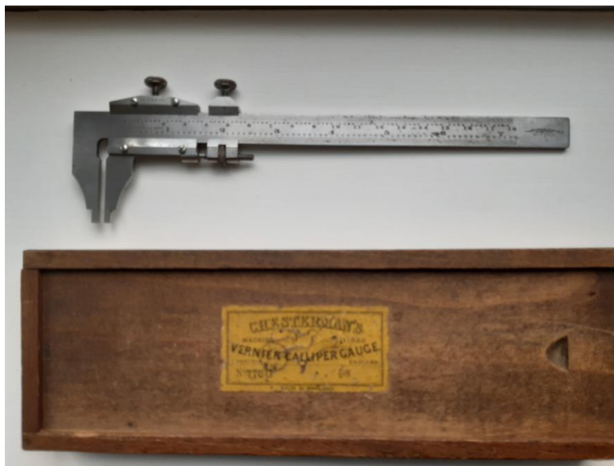
A Chesterman's Vernier Calliper Gauge which belonged to Les Buckett and was used to check the dimensions of pieces being manufactured.
